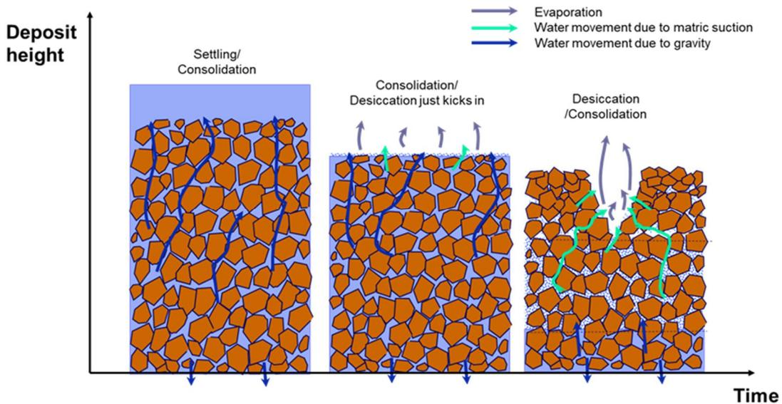
Figure 3 Sketch of driving forces expelling water out of the deposit during different ripening phases.
