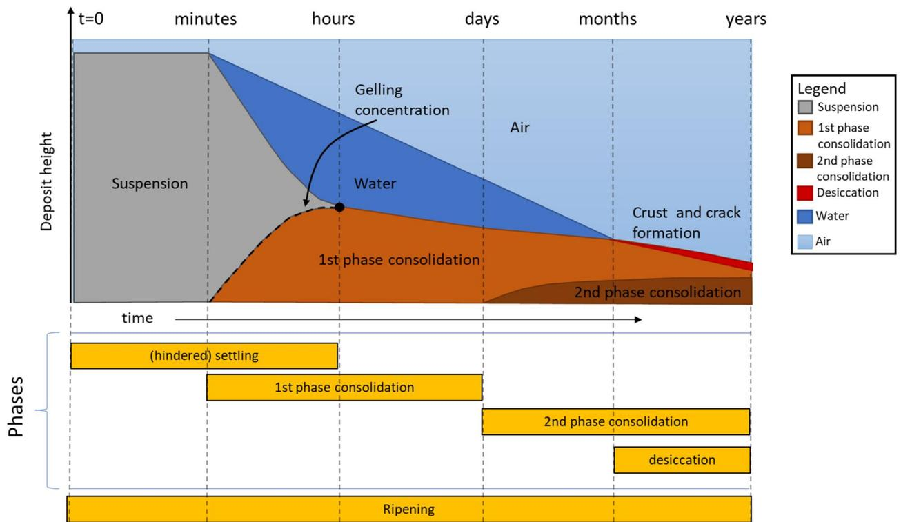
Figure 2 Schematic representation of the ripening process, indicating the different phases and their chronology. Associated timescales for the different phases are also indicated. Adapted from Talmon et al. (2018)
