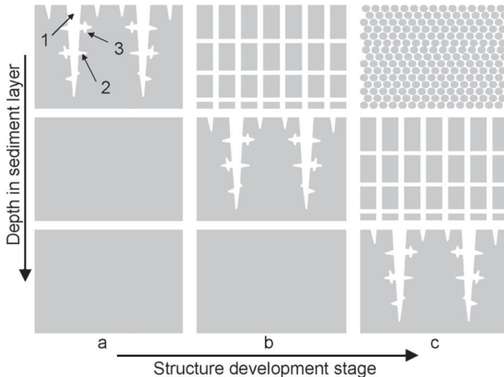
Fig. 2.2: Schematic cross section of a layer of dredged material at different, stages of structure development (After Baver et al. 1972, Dexter, 1988 and, Vervoort et al. 1999). a = very coarse prismatic structure with primary (1), secondary (2), and tertiary cracks (3); b = coarse blocky and platy aggregates on very coarse prismatic structure; c = medium and fine aggregates on coarse blocky and platy aggregates and very coarse prismatic structure
