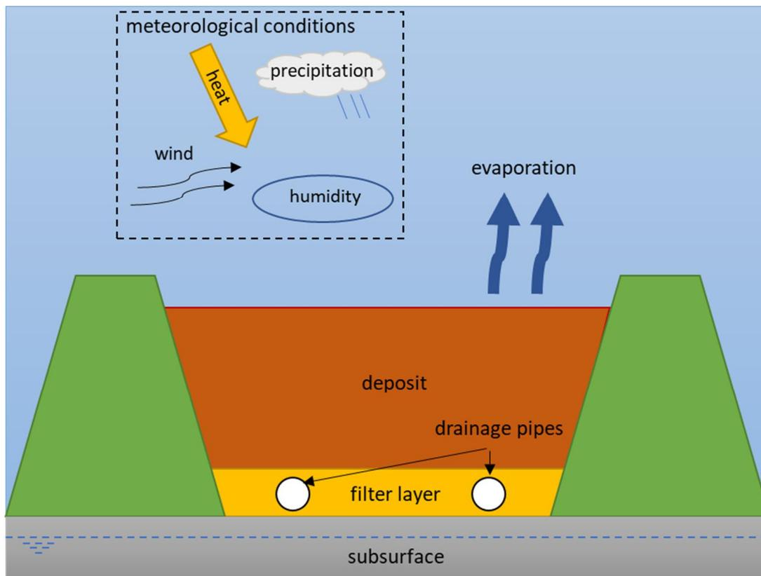
Figure 5: Conceptual sketch of desiccation phase. Top part of deposit is not (fully) saturated, air can penetrate deposit. Water evaporates from top layer, rate at which this happens depends on climatic conditions and properties of deposit.
