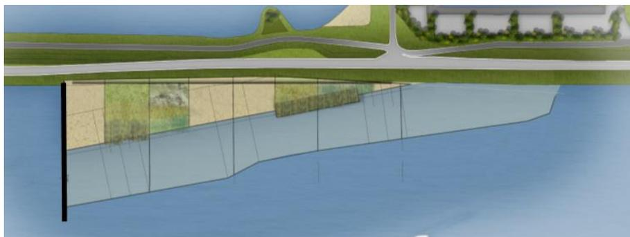
Figure 2 Lay-out of the pilot section with four sections of each 100 m width and each section planted manually, while the other half is left to develop on its own. The willow faggots mattress is positioned in the right-hand smaller section.
