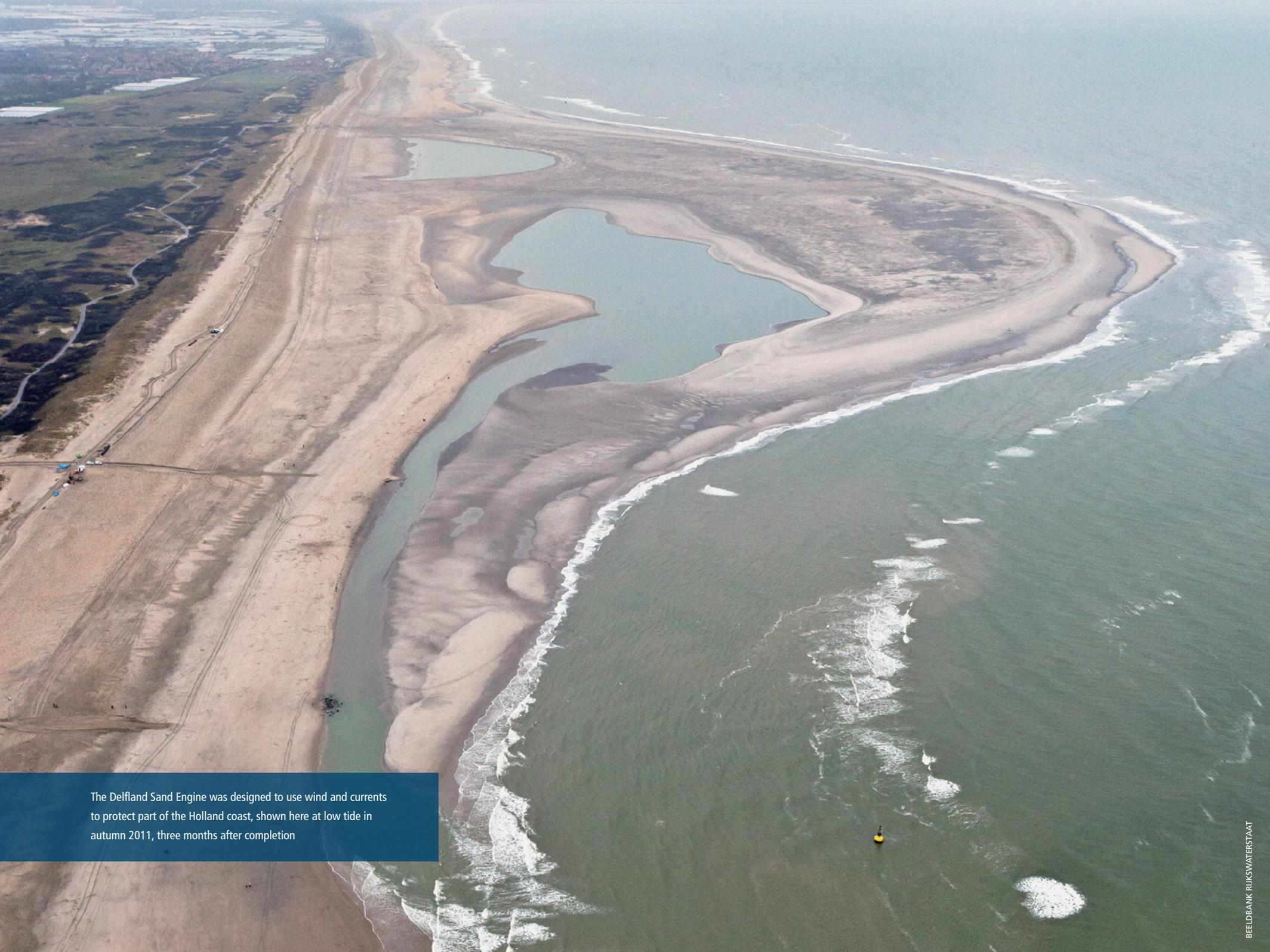
The Delfland Sand Engine was designed to use wind and currents to protect part of the Holland coast, shown here at low tide in autumn 2011, three months after completion
