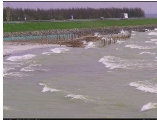
Photos made by the camera at the pilot location on 12 September 2014, with the first reeds on a braided brushwood mattress (left), and on 11 April 2015, showing a marked effect of the waves on the braided brushwood mattresses (right). Parts of the braided brushwood mattresses were washed away during the winter of 2014-2015. The planted reeds can be seen behind the mattresses.
