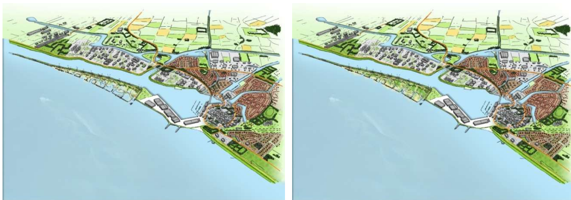
Figure 5. Proposed lay out of the pioneer salt marsh at the start (left, only pioneer zone) and expected size around 2060 (right, full range from pioneer zone to developed salt marsh) (Dankers et al, 2013).
