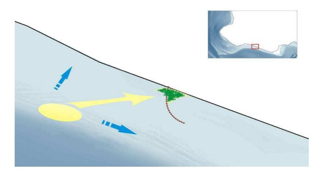
Figure 3; 'soft sand engine'. Proposal to deposit sand in the lake and let the waves transport the sand to the coast where new flood plains emerge. The wooden poles in the picture break the wave energy.
