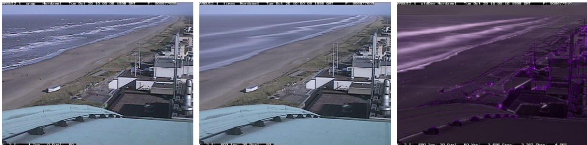
Figure 5: The Argus system three types of images, station Egmond, The Netherlands (left to right: snapshot, time exposure and variance image)
