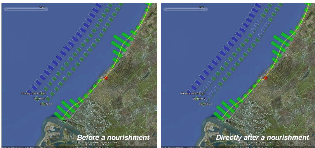
Figure 5d: Coastal development and coastal indicators for reference scenario 4 (Seaward). Moments in time before and after a nourishment took place.
