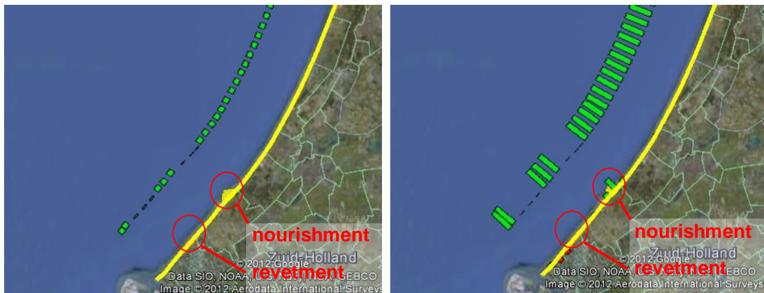
Figure 3: Ecological indicator for the impact of coastal measures on the benthic population (bars shown at 10 km offshore) and the current coastline (yellow line) after one year (left panel) and seven years (right panel).
