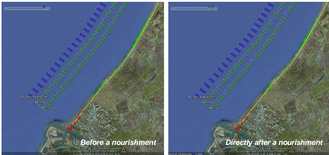
Figure 5c: Coastal development and coastal indicators for reference scenario 3 (Minimal consolidation: Five yearly nourishments). Moments in time before and after a nourishment took place.
