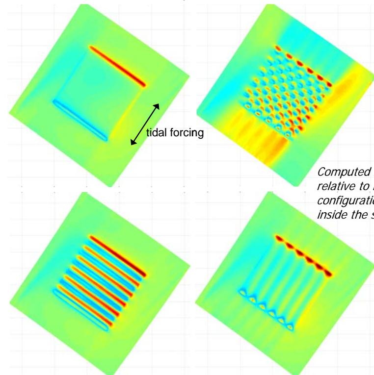
*Computed bed shear stress relative to flat bed case for four configurations of the sea bed inside the sand mining pit*
