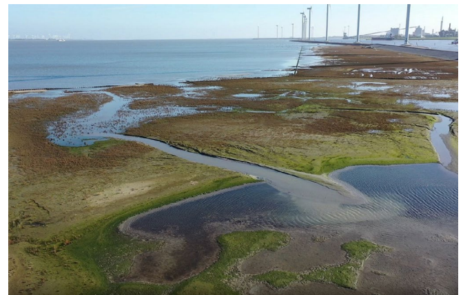
Figure 1: The Marconi salt marsh project, adding value by enriching a hard sea defense with a vegetated foreshore.
