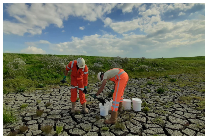
Figure 4: Ripening dredged sediment for dikes at the Clay Ripening Pilot Project.
