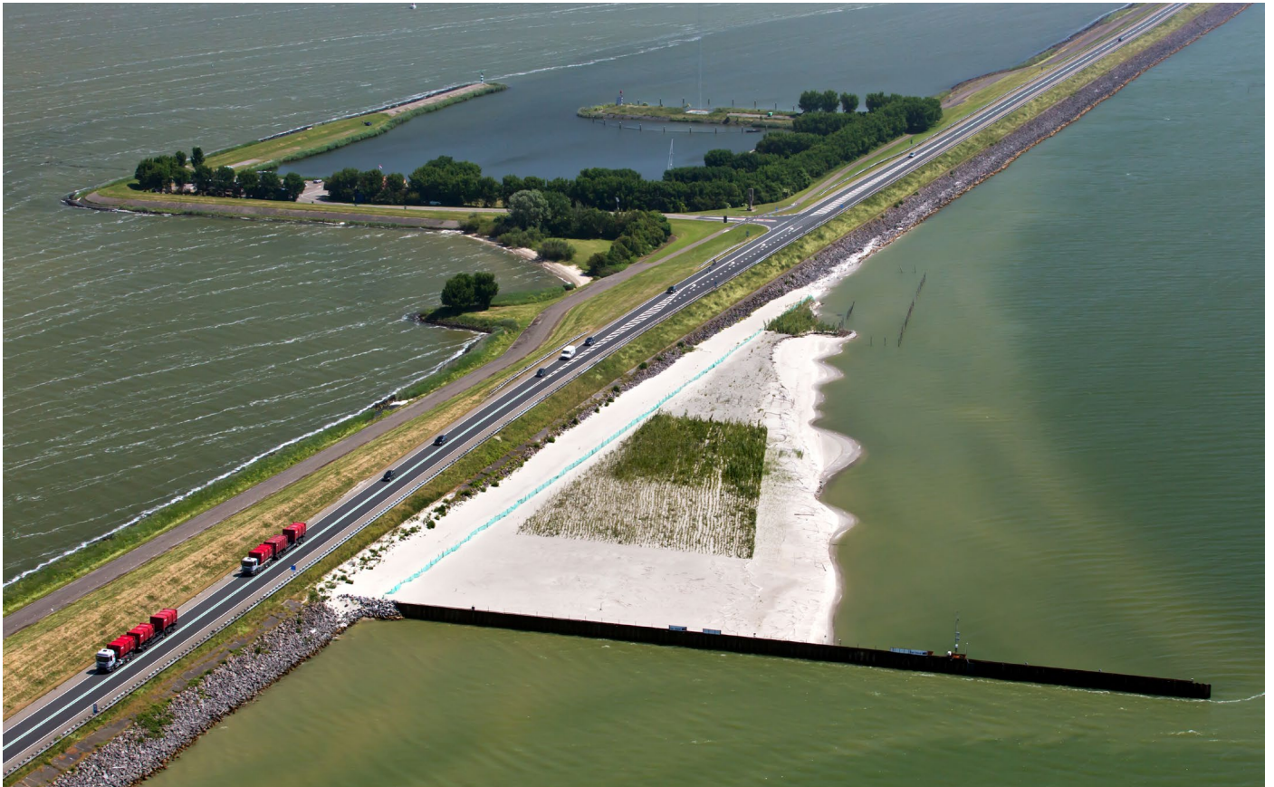
Figure 5: The Houtribdike Pilot Project investigated the behavior of a vegetated foreshore in a lake environment, resulting in upscaling of the concept.
