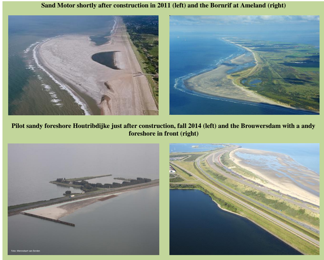
Figure 3. On the left hand side the Ecoshape sandy pilots Sand Motor (upper) and Sandy foreshore Houtribdijk (lower) and on the right similar already existing solutions in other environments
