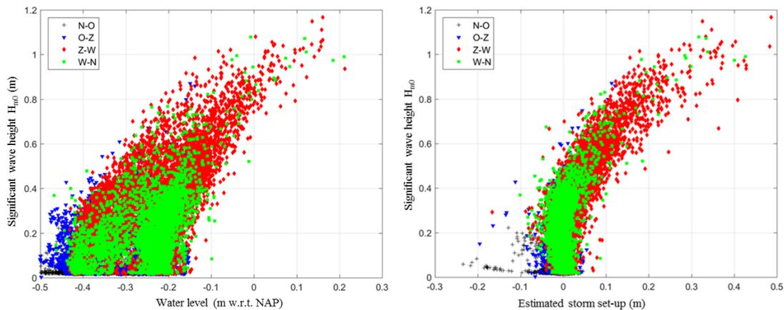
Figure 11a Overview of all combinations of water level and wave heights; Figure 11b Overview of all combinations of the estimated storm set-up and wave heights all for four sections of wind direction.
