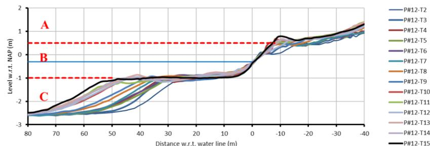
Figure 12 Development of the cross-shore profile shape at location 12, plotted relative to the intersection with the NAP-0.3 m level. Including the definition of the upper (A), middle (B) and lower layer (C).
