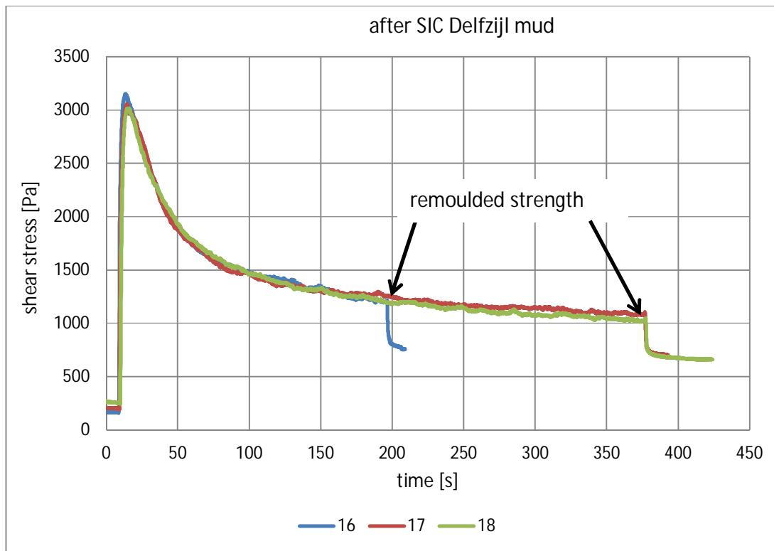
Figure 4.7 Results from the vane tests performed on the sample after the SIC was finished
