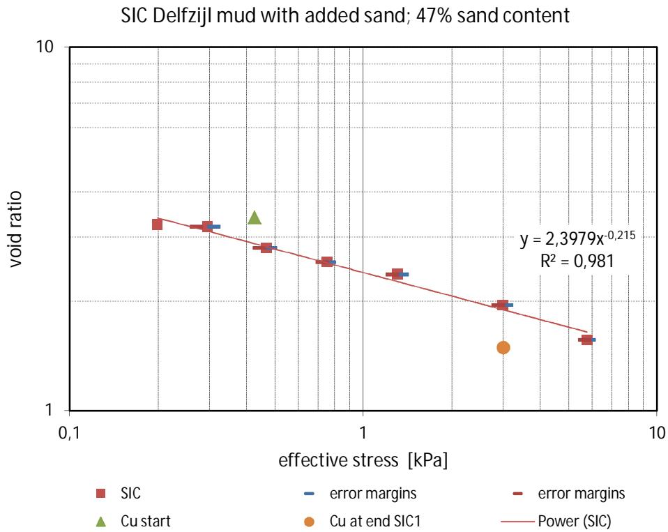
Figure 4.3 Void ratio as function of effective stress for sample SIC
