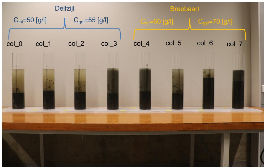
Figure 2.1 shows eight columns used for the main column tests in this study; in this image column number is in black; the initial concentration and gelling concentration of mud from Delfzijl and Breebaart is in blue and orange, respectively. Image is taken at August 21, 2017, 17:49:17, about an hour after the initiation of the experiment.
