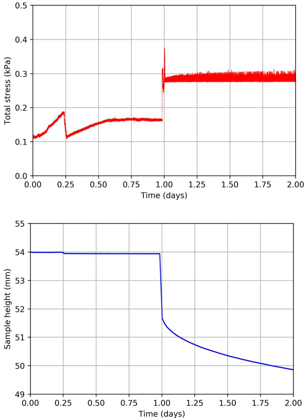
Figure 4.9 First loading step and part of second loading step for SIC on Delfzijl mud: (above) in total applied vertical stress and (below) the change in sample height
