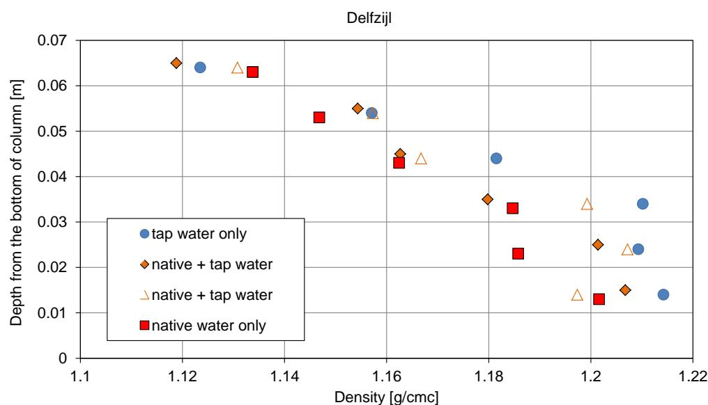
Figure 3.7 Density profile along the depth of those columns with mud from Delfzijl at the end of the experimental period (93 days after the initiation of experiment).
