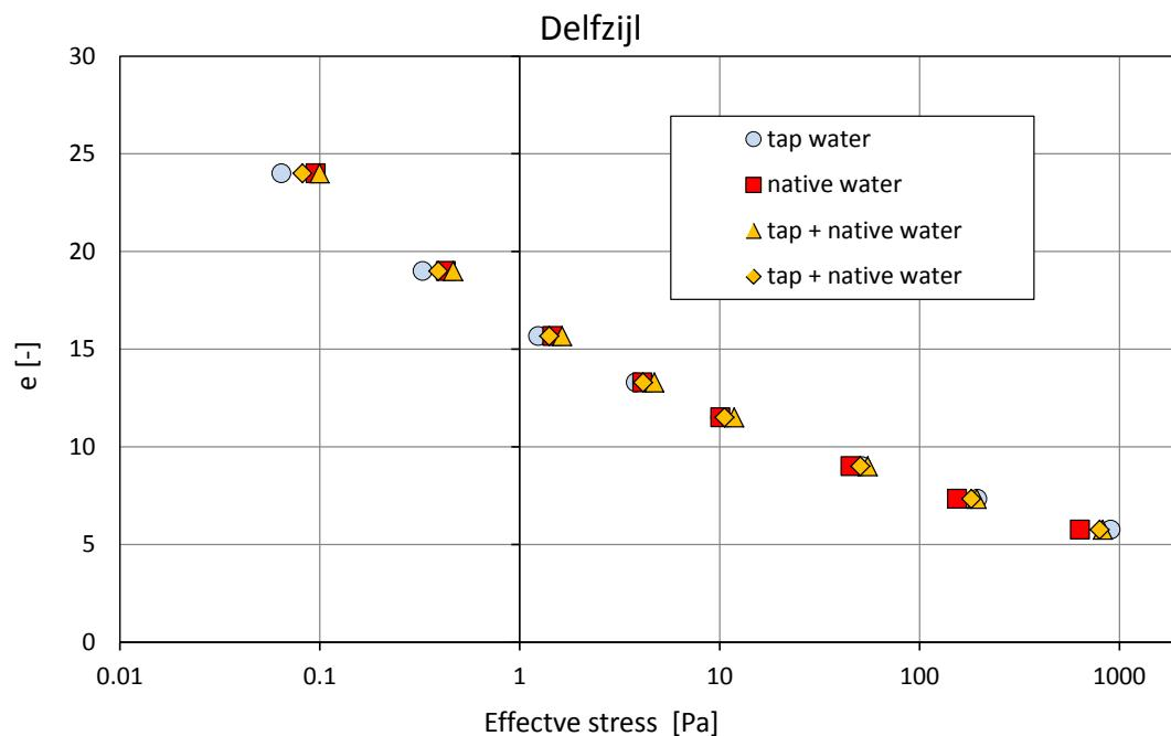
Figure 3.5 Relationship between  $e$  and effective stress for mud from Delfzijl for different salinity levels.
