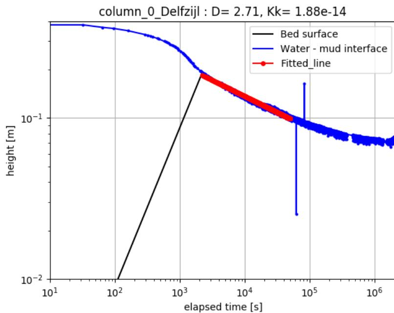
Figure 2.3 Temporal evolution of settling curve for test id col\_0 (mud from Delfzijl) on a log-log scale.
