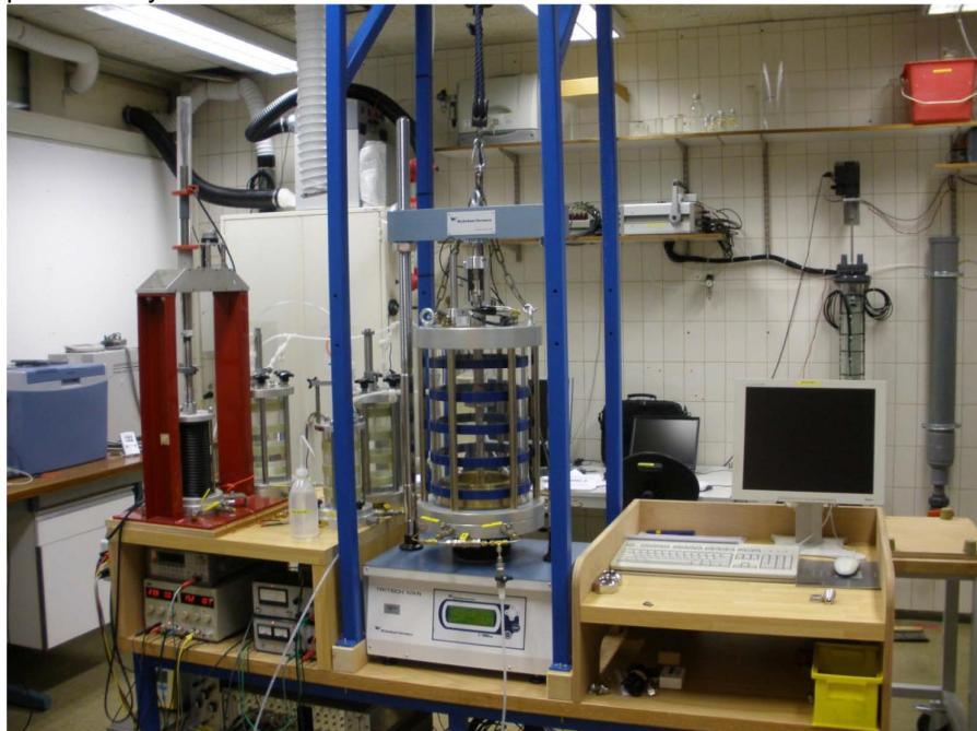
*Figure 2.1 Photo of the SIC apparatus at Deltarès. The sample holder is in the lower part of the cell. Underneath the cell, the motor controls the imposed external load by controlled displacement of the sample against the fixed piston inside the cell. To the left of the cell the automatic pump is for pore water suction and to the right the computer for test control and data storage*
