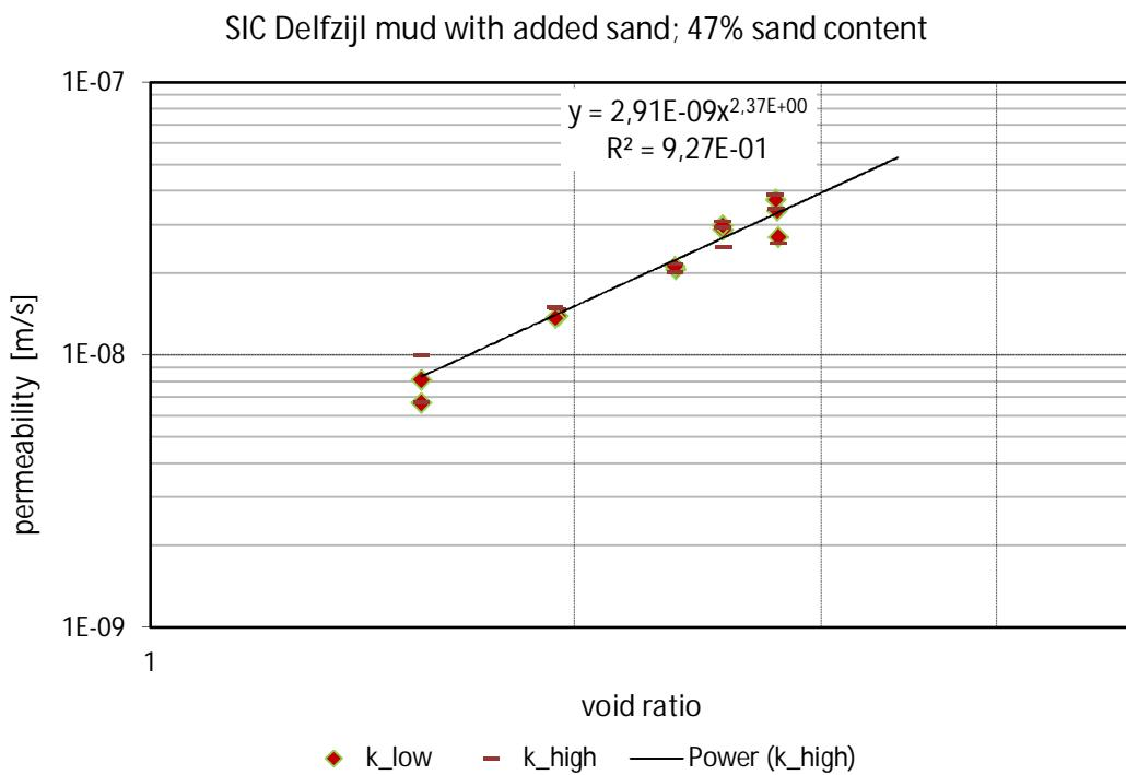
Figure 4.2 Permeability as function of void ratio for sample SIC
