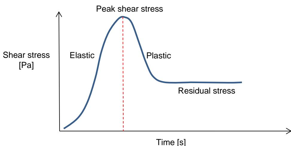
Figure 2.2 A schematic view of shear stress development with time.
