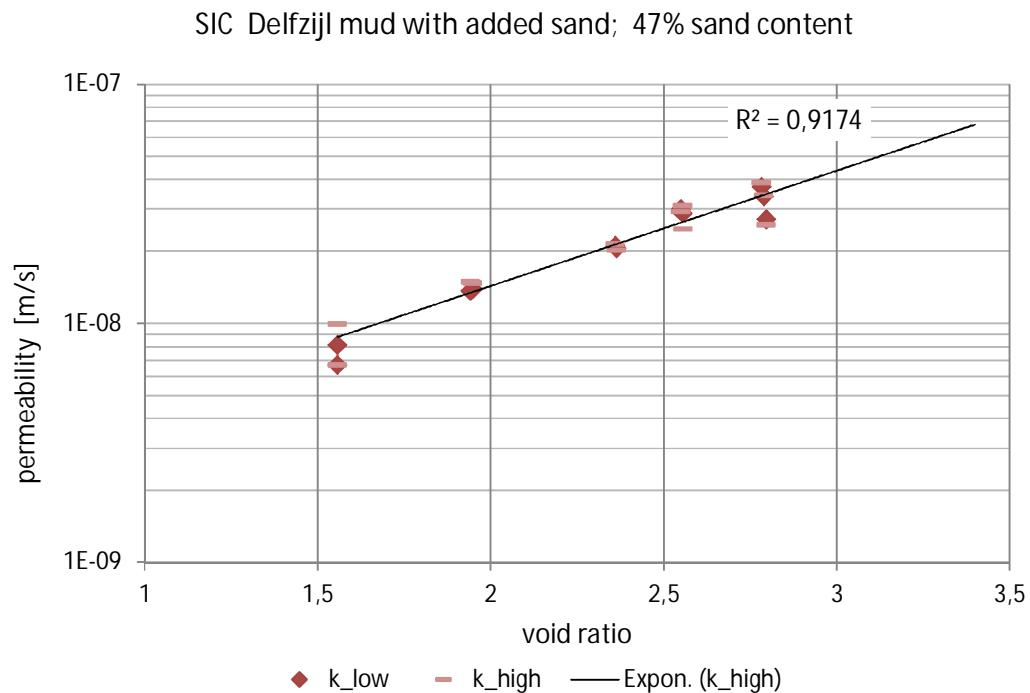
Figure 4.4 Permeability as function of void ratio for sample SIC
