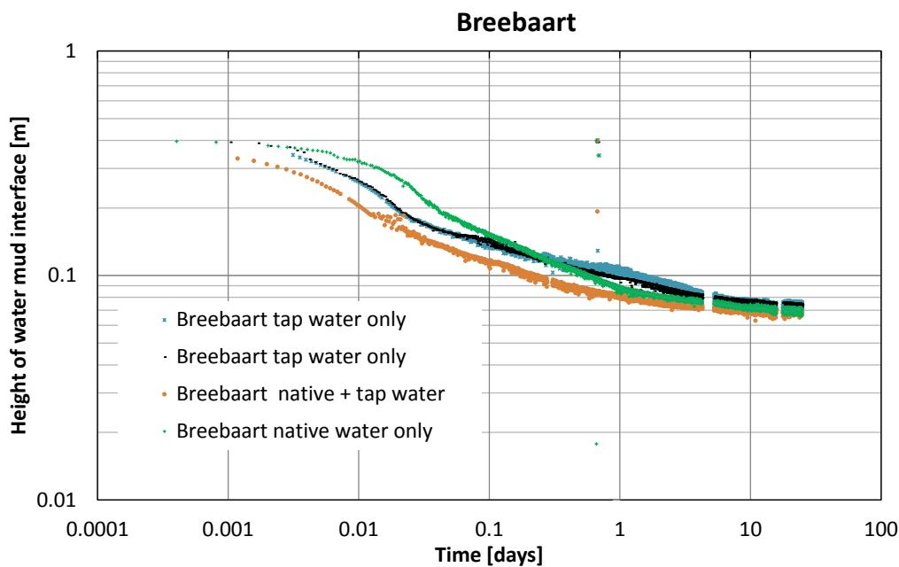
Figure 3.2 The settling curves of mud from Breebaart from the initiation of the experiment until day 25 for different salinity levels on a log-log scale.
