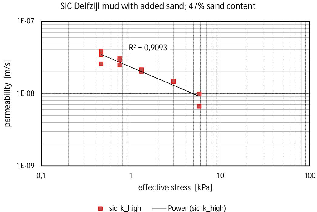
Figure 4.1 Permeability (upper limit) as function of effective stress for sample SIC
