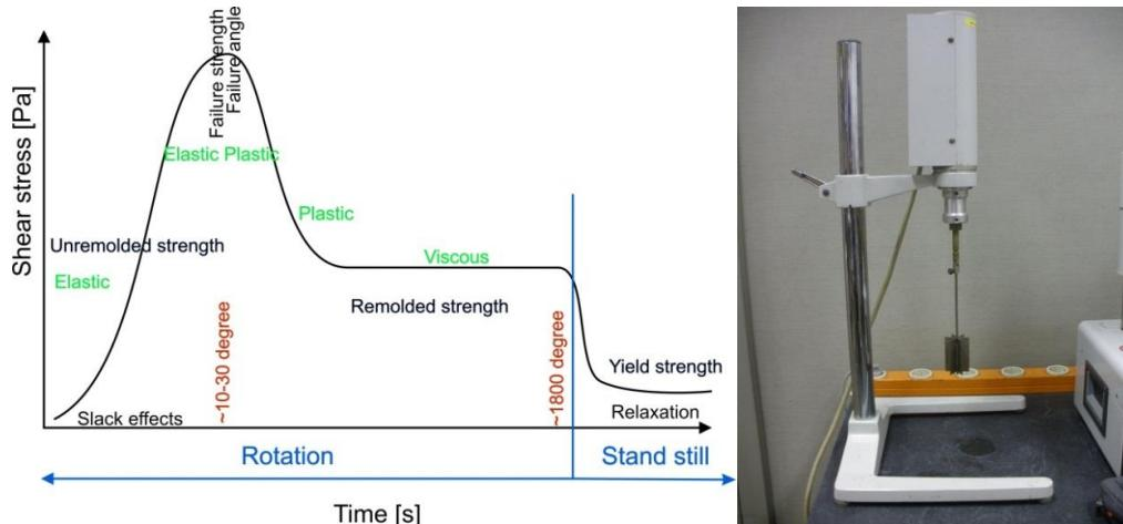
Figure 2.3 Vane results schematization (left) and Vane apparatus (right)
