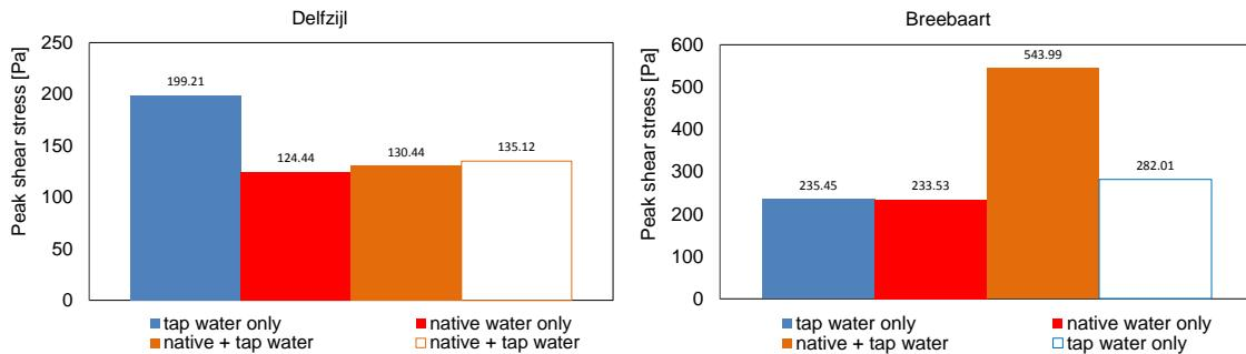
Figure 3.10 Strength (peak shear stress at 0.5 RPM rotation speed) measured at 2.5 cm below the water - mud interface of mud from Delfzijl (graph at left) and from Breebaart (graph at right) at the end of the experimental period (93 days after the initiation of experiment).
