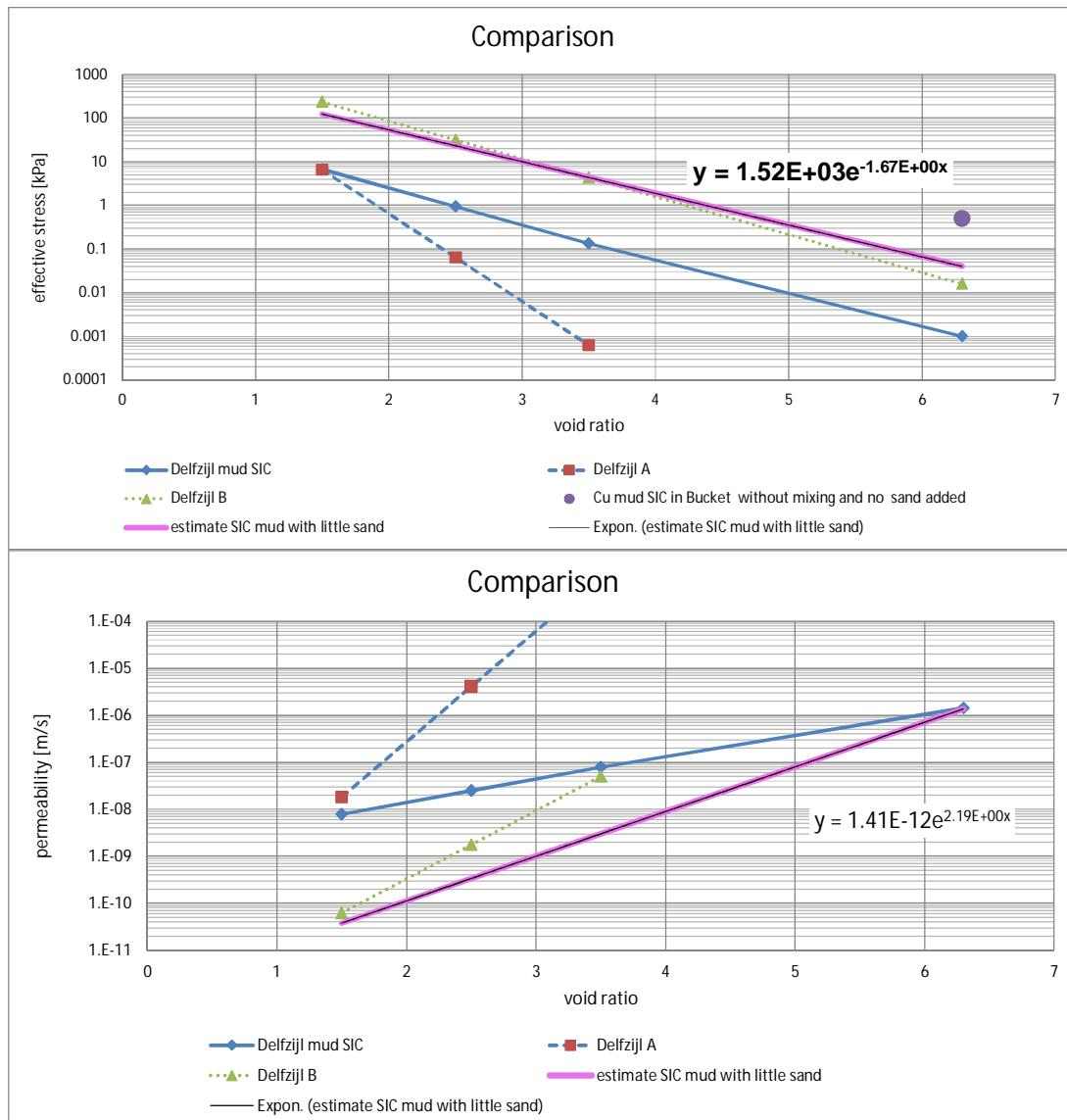
Figure 5.1 The effective stress – void ratio (above) and permeability – void ratio (below) relations for the Delfzijl mud type in Table 5.1. The 'Delfzijl mud SIC' indicates the SIC sample (sand content 47%). The pink lines are the estimates for Delfzijl mud from Harbour section 3 (sand content 1%)
