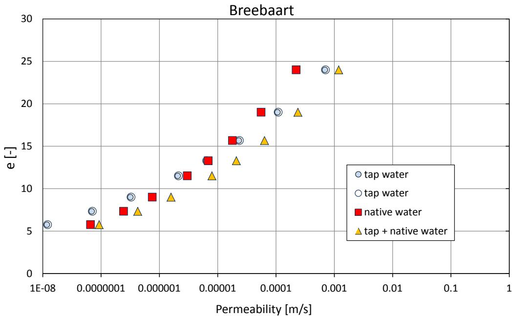
Figure 3.4 Relationship between  $e$  and permeability for mud from Breebaart for different salinity levels.
