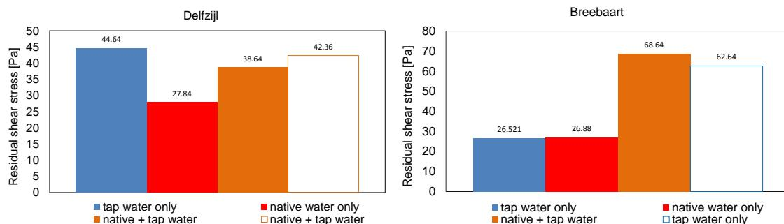
Figure 3.11: Strength (residual shear stress at 0.5 RPM rotation speed) measured at 2.5 cm below the water - mud interface of mud from Delfzijl (graph at left) and from Breebaart (graph at right) at the end of the experimental period (93 days after the initiation of experiment).
