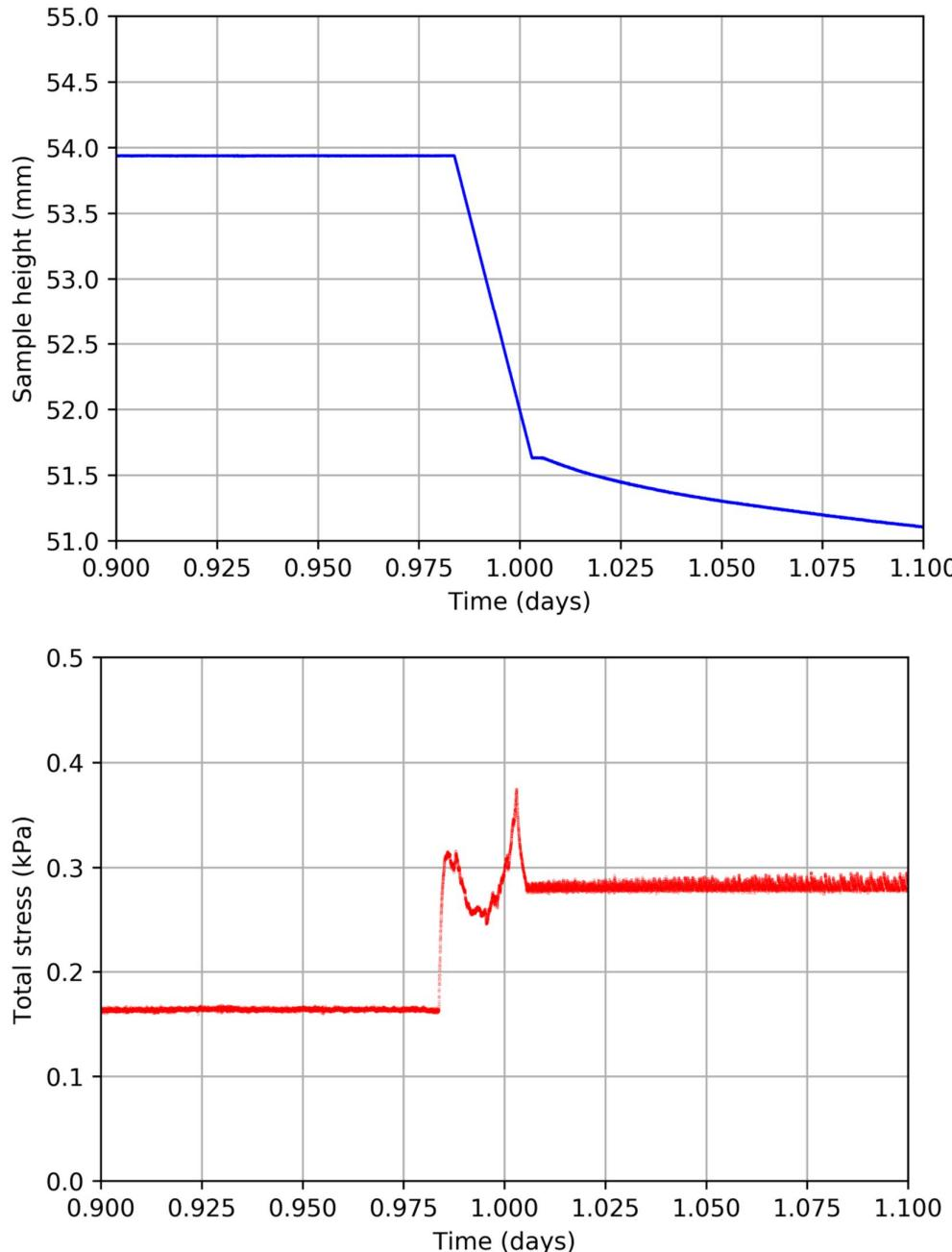
Figure 4.10 Detail of SIC on Delfzijl mud: (above) loading at constant displacement speed at the end of the first loading step; part of the second loading step is also shown; (below) the resulting change in applied total vertical stress
