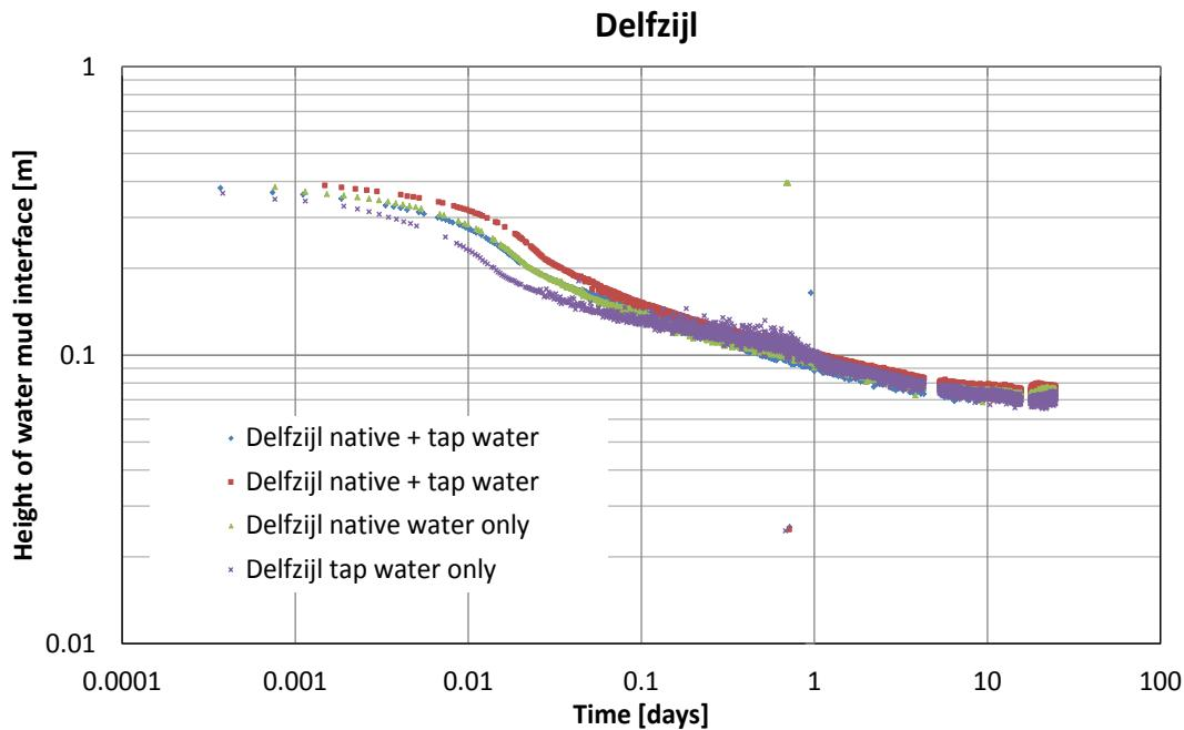
Figure 3.1 The settling curves of mud from Delfzijl from the initiation of the experiment until day 25 for different salinity levels on a log-log scale.
