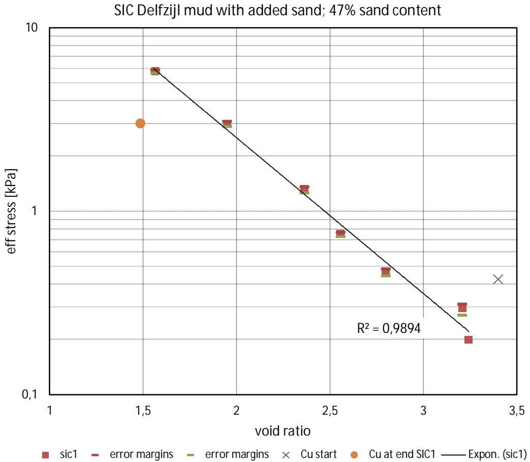
Figure 4.5 Effective stress as function of void ratio for sample SIC
