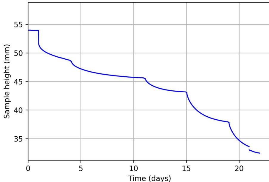
Figure 4.8 Loading steps for SIC on Delfzijl mud: (above) in total applied vertical stress and (below) the resulting changes in sample height
