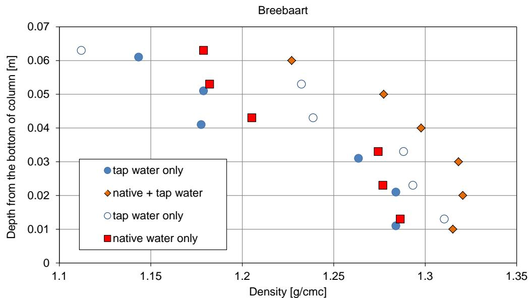
Figure 3.8 Density profile along the depth of those columns with mud from Delfzijl at the end of the experimental period (93 days after the initiation of experiment).
