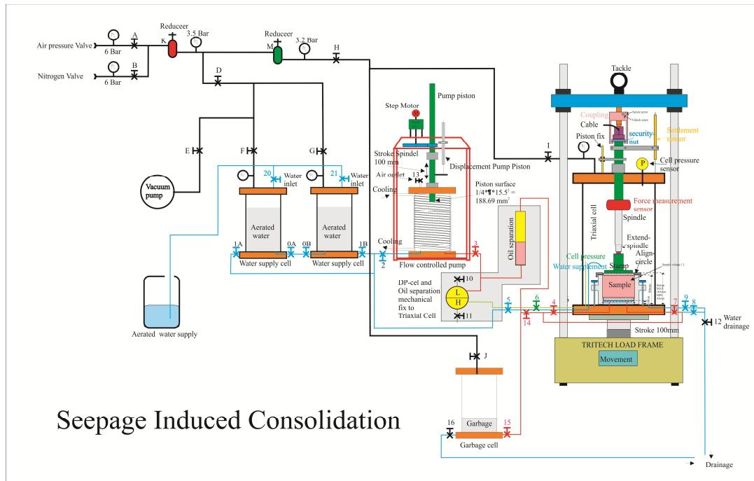
Figure 2.2 Schematic flow diagram of the SIC apparatus
