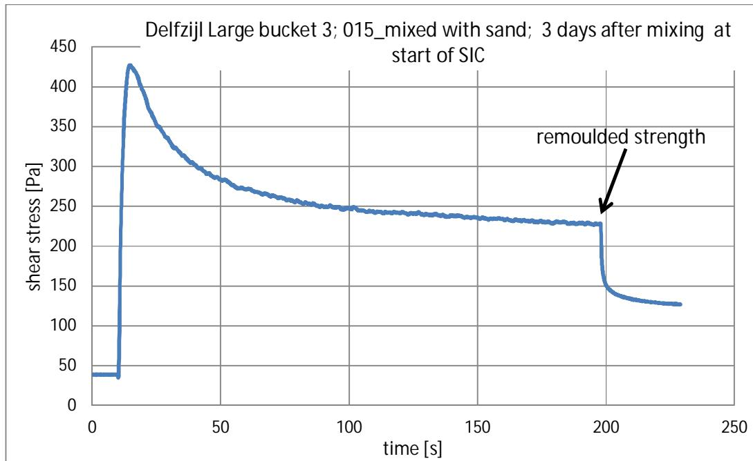
Figure 4.6 Results from vane test that was performed 3 days after mixing, i.e. at the time the loading started for the SIC
