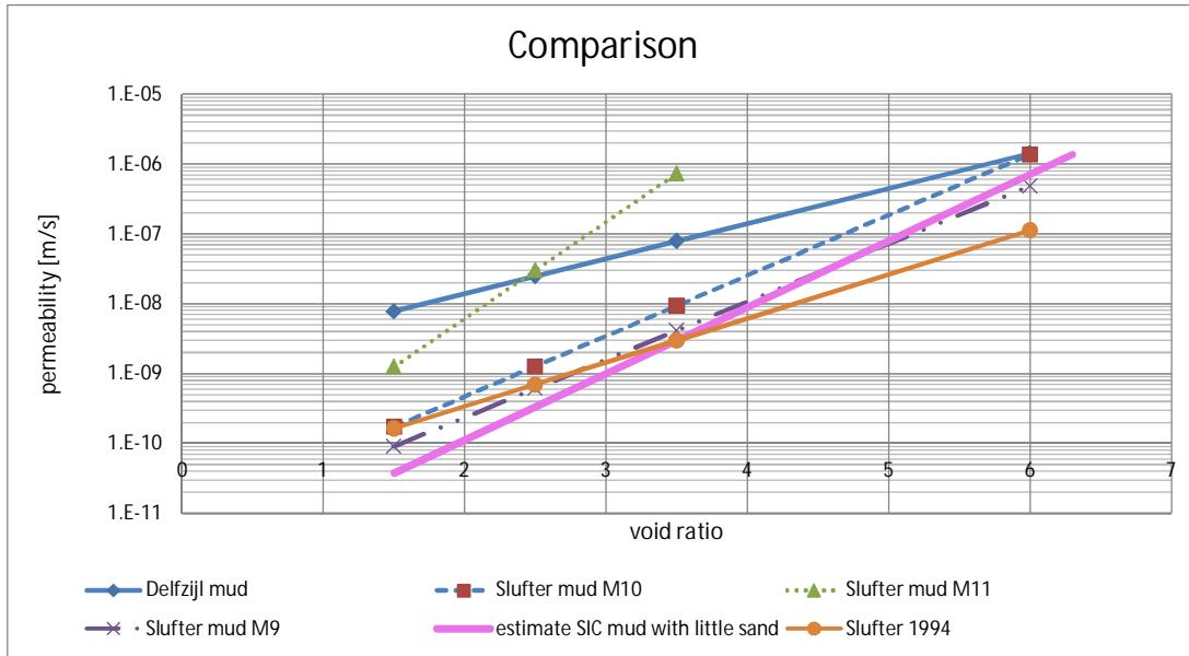
Figure 5.2 The effective stress – void ratio (above) and permeability – void ratio (below) relations for the Slufter mud type in Table 5.1. The ‘Delfzijl mud’ indicates the SIC sample (sand content 47%). The pink lines are the estimates for Delfzijl mud from Harbour section 3 (sand content 1%)
