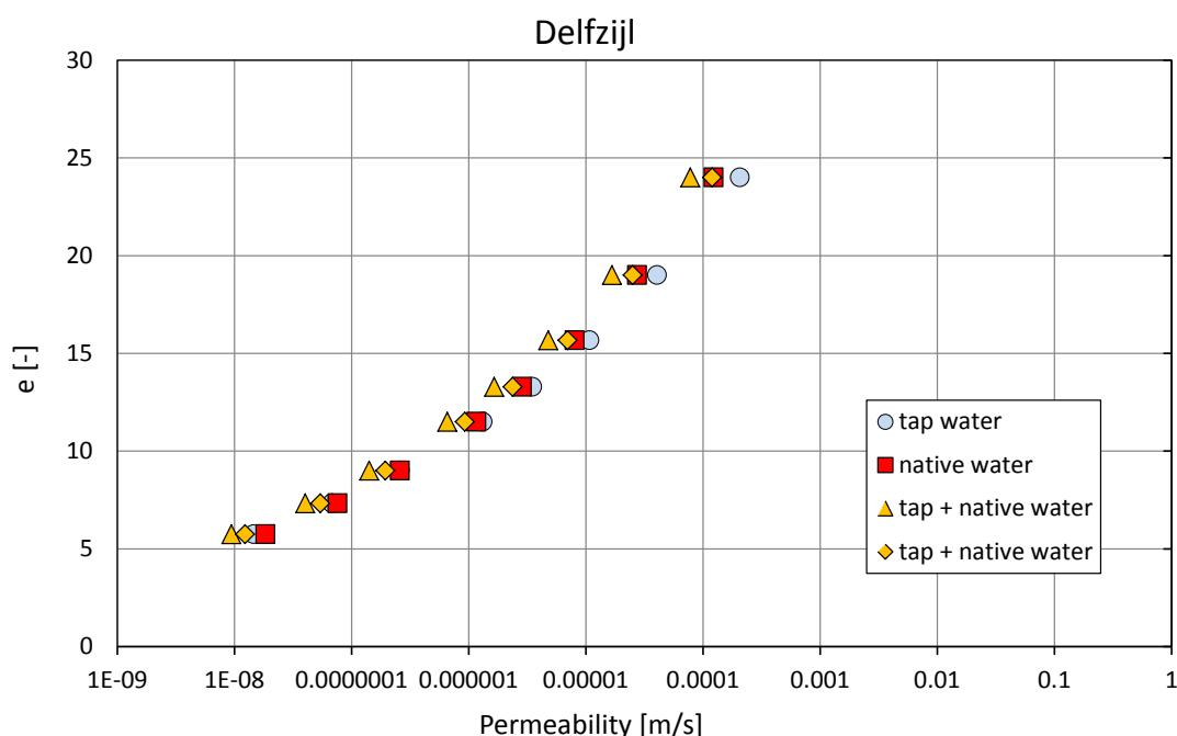
Figure 3.3 Relationship between  $e$  and permeability for mud from Delfzijl for different salinity levels.
