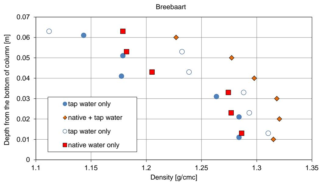
Figure 3.9 Density profile along the depth of those columns with mud from Breebaart at the end of the experimental period (93 days after the initiation of experiment).
